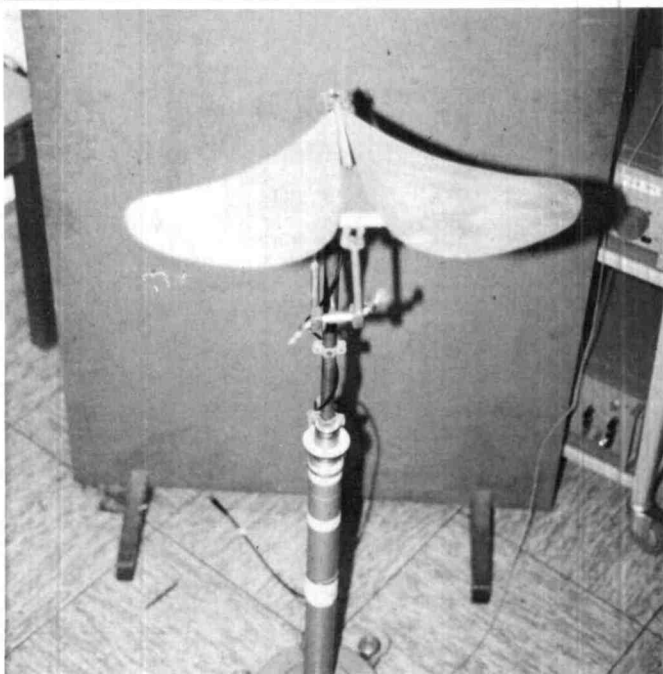
Common materials can be used to build the antenna. Here you see the Heart antenna made of aluminum sheet stock.
