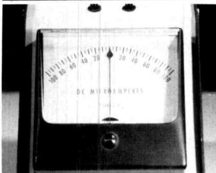
Zero center meter movement.
