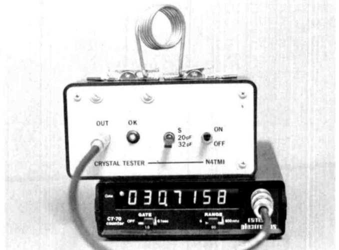
To test a coil, measure resonant frequency with 32 pF.
